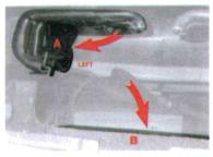
3. Insert the paddles (A) into the cut ducts, using the "U" section to guide the correct position. Remove backing paper and the stick the foam block (B) in central position as shown.
